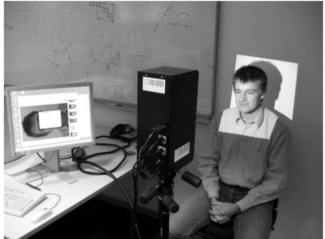
Fig. 1. Active acquisition device for three-dimensional face scanning
